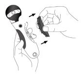
Remove the 4 screws using a Phillips-head screwdriver. Remove the upper body of handle to change the button/blade, guard/spring, etc...
