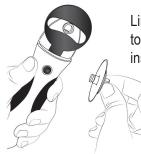
Line up the flat edge of the stem to the flat edge of the hole and insert the stem into the hole.
