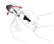
While holding the button down, slide the lever left or right to move the blade cover.
