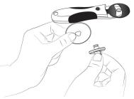
Remove the old blade and replace it with the new one.
