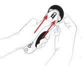
While holding the stem into place, slide the lever up to lock the blade into place.
